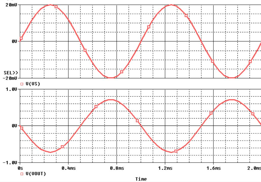
5. VS and V<sub>OUT</sub> for  $B_f=150$  are shown below
