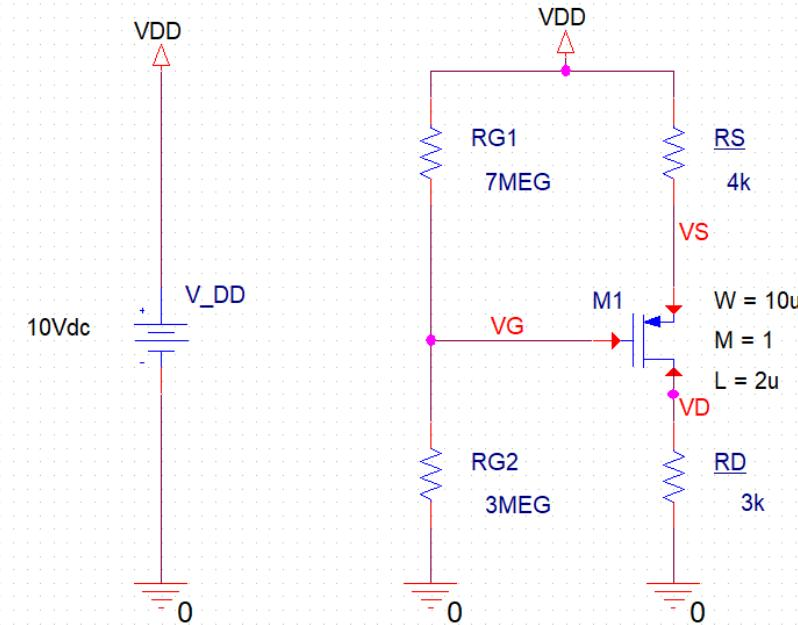
2. The transistor used here has  $k_n' = 100 \mu\text{A}/\text{V}^2$ . So,  $\text{W/L} = 10\mu/2\mu$  is chosen to get  $k_n = 0.5 \text{ mA/V}^2$ .
