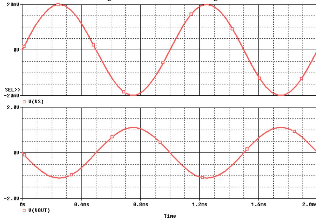
4. To find the variation in gain, change  $B_f$  to 50 and 150 and repeat the simulation. VS and V<sub>OUT</sub> for  $B_f=50$  are shown below
