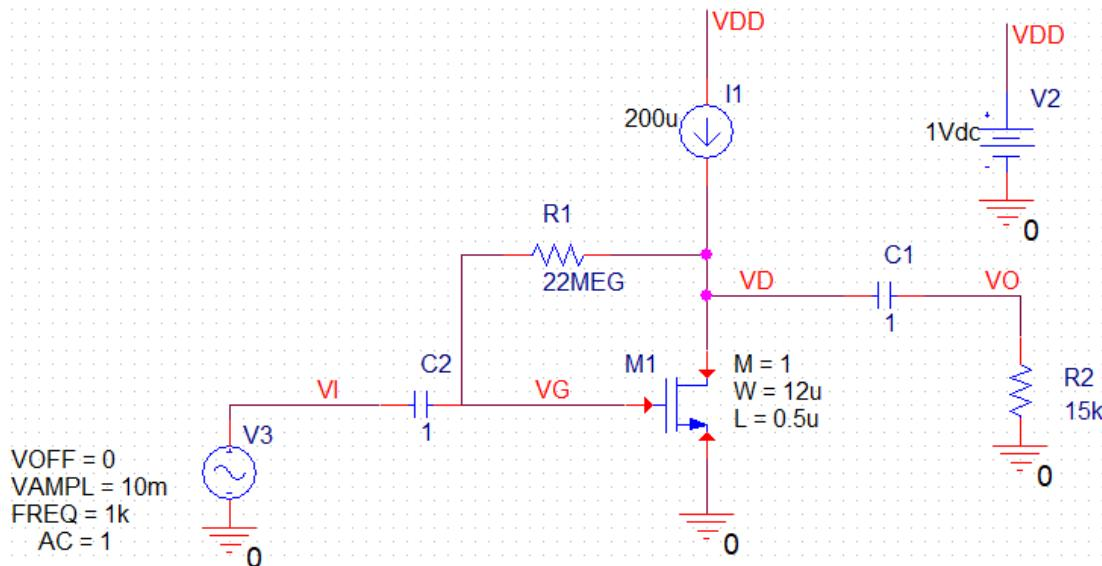
2. Run the netlist and perform AC simulation. Plot  $DB(V(VO)/V(VI))$  to get the gain.
