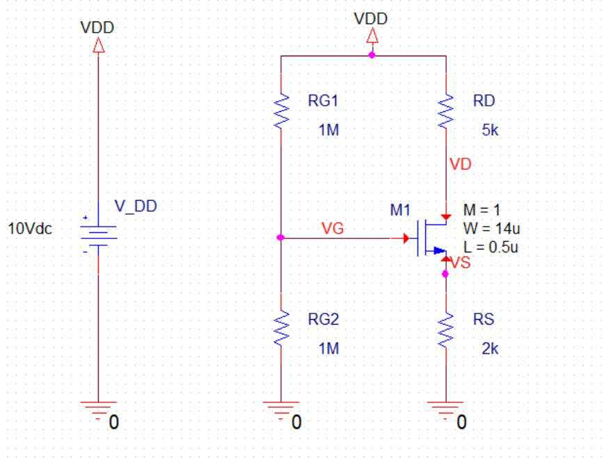
2. The transistor used here has  $k_n' = 71.2 \mu\text{A}/\text{V}^2$ . So,  $\text{W/L} = 14\mu/0.5\mu$  is chosen to get  $k_n = 2 \text{ mA}/\text{V}^2$ .
