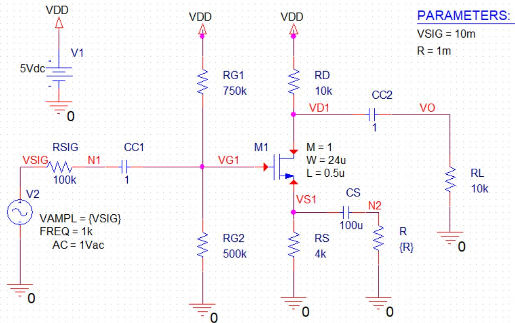
2. The transistor used here has  $k_n' = 167.2 \mu\text{A}/\text{V}^2$ . So,  $\text{W/L} = 24\mu/0.5\mu$  is chosen to get  $k_n = 8 \text{ mA}/\text{V}^2$ .
