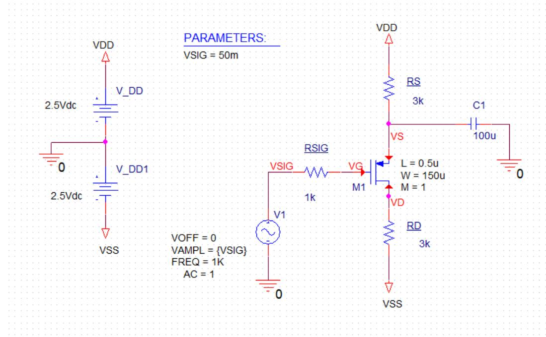
2. For part (a), run the netlist and find the operating point.
