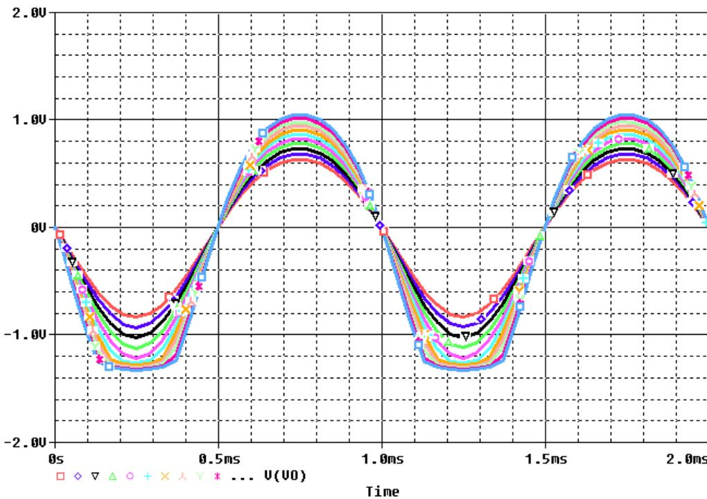
8. The output starts to saturate when input has an amplitude above 0.15 V.
