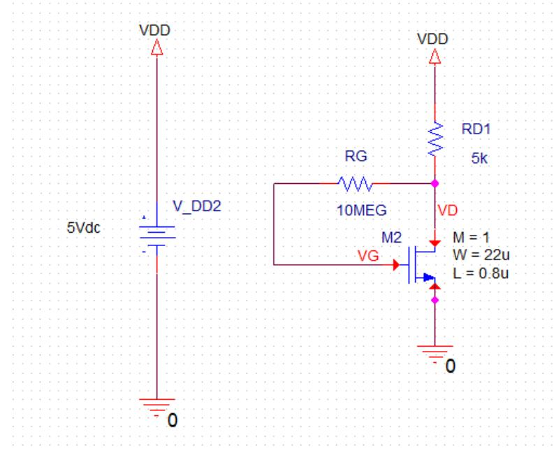
2. The transistor used here has  $k_n' = 181.7 \mu\text{A}/\text{V}^2$ . So,  $\text{W/L} = 22\mu/0.8\mu$  is chosen to get  $k_n = 5 \text{ mA}/\text{V}^2$ .
