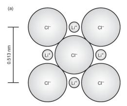
Calculation using Pythagoras' Theorem gives the length of the diagonal as 0.725 nm, which gives the atomic radius  $r_{\text{Cl}}$ - as 0.18 nm (1.8 Å).
